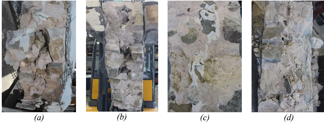
Figure 14. Detail of the cross section of the samples after the tests: (a) sample S_I-MA_B200; (b) sample S_I-MA_B400, (c) sample S_I-MA_S600, (d) sample S_I-MA_B200-S600.
