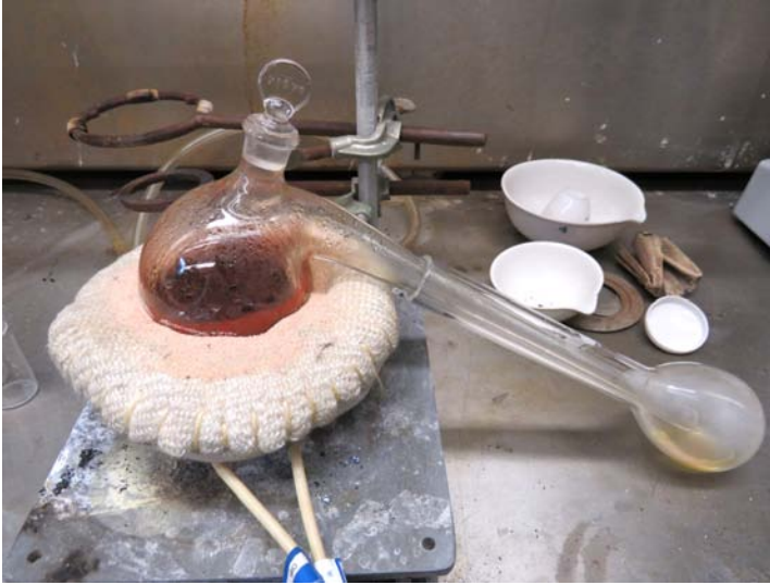
FIGURE 5 Distillation of the golden ink mentioned in recipe No. 10, interpreting talq as silica. Baltimore, Johns Hopkins University, Department of History of Science and Technology, 14 September 2018
