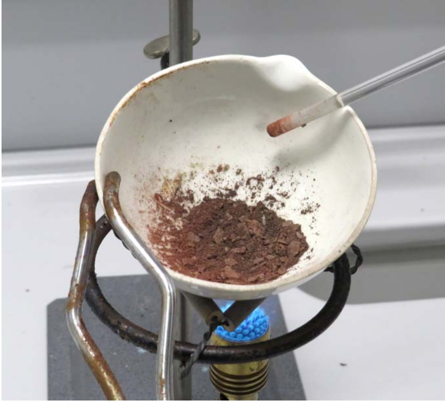
FIGURE 4 Red vitriol obtained after the calcination of green and blue vitriol. Bologna, Dipartimento di Chimica 'Giacomo Ciamician', 6 February 2019 PHOTO: LUCIA RAGGETTI
