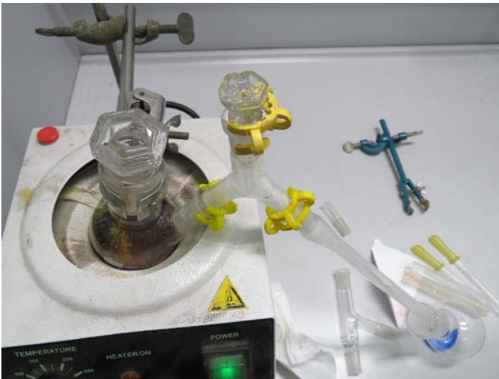
FIGURE 6 Distillation of the golden ink mentioned in recipe No. 10, interpreting talq as slaked lime. Bologna, Dipartimento di Chimica 'Giacomo Ciamician', 6 February 2019
