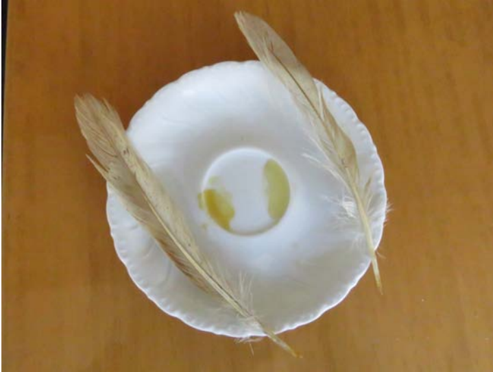
FIGURE 11 The products of the two different distillations directly mixed with gum arabic; on the right, the version containing slaked lime; on the left, the version containing silica—along with the chicken feathers used for the writing test. Bologna, 4 April 2019 PHOTO: LUCIA RAGGETTI
