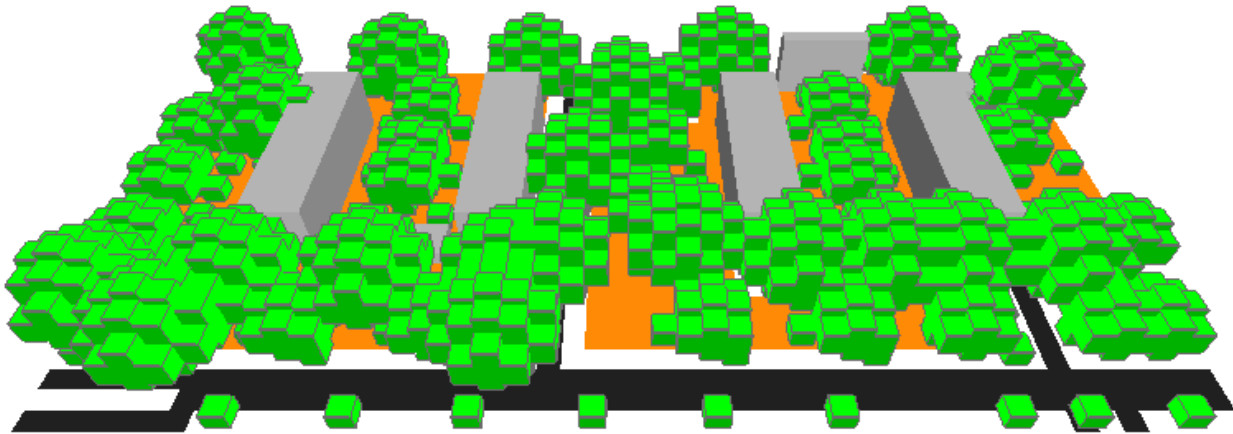
Figure 57 A 3-dimensional picture from the ENVI-met tool 'SPACE' of the Myyrmäki Vaskivuorentie area; grey: buildings, light green: trees with different heights and shading areas, orange: unsealed loamy area, not vegetated; white: sealed areas, stone slabs, black: main sealed roads with tarmac.
