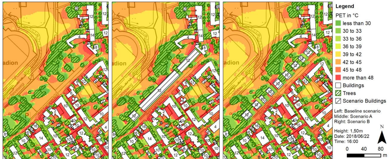
Figure 38 Model Bottrop 'Am Lamperfeld' – ENVI-met calculated PET (source: own account, data: City of Bottrop)
