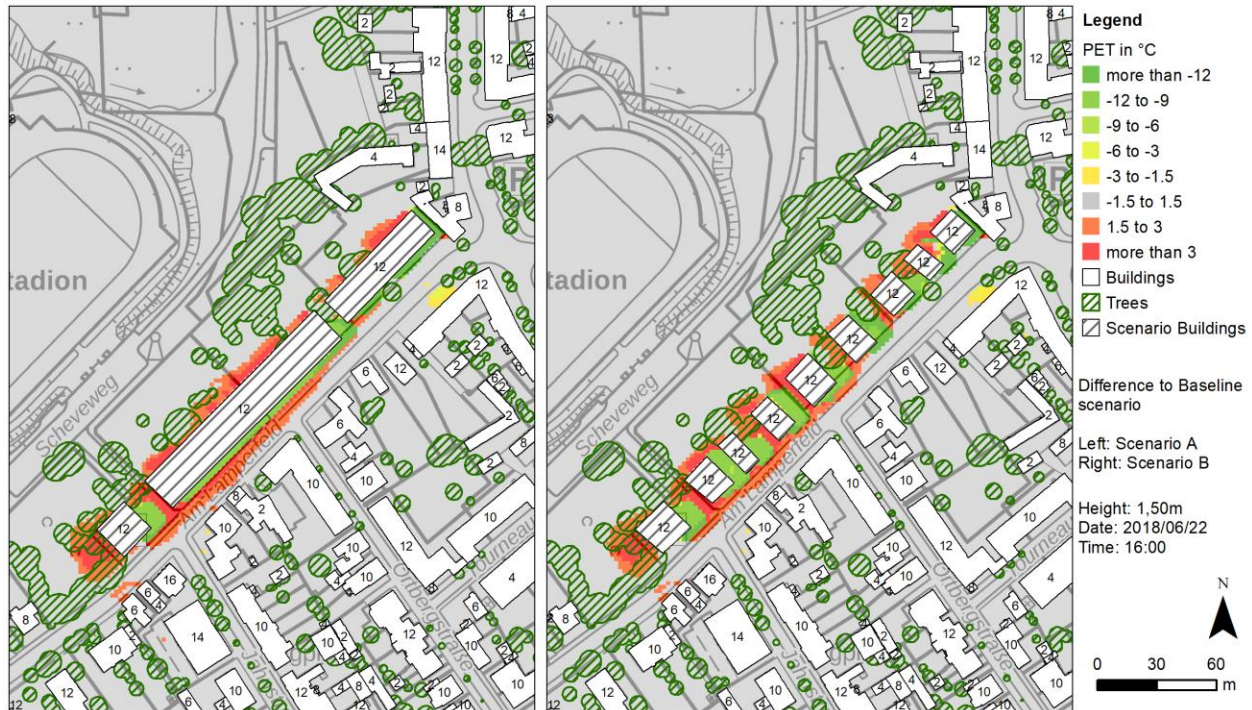
Figure 39 Model Bottrop 'Am Lamperfeld' – Difference of PET, scenario A/B minus baseline scenario (source: own account, data: City of Bottrop)
