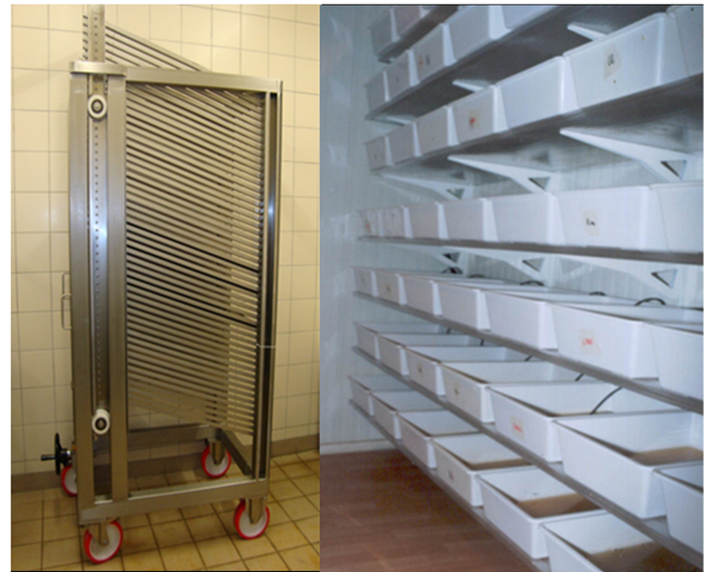
Figure 1. FAO/IAEA larval rearing unit (left) and standard laboratory trays used for Aedes albopictus larval mass rearing procedures (right).
