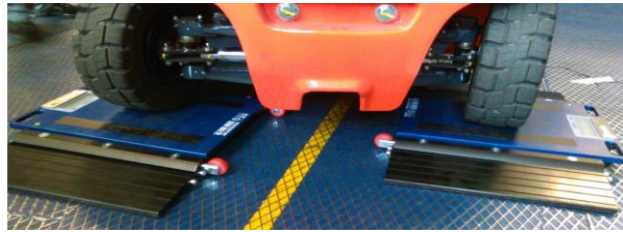
Fig 4. Close up of the load cells in Test 3 .
