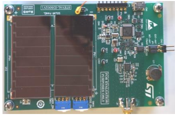
Figure 3. Power Unit board equipped with the PV harvesting system.
