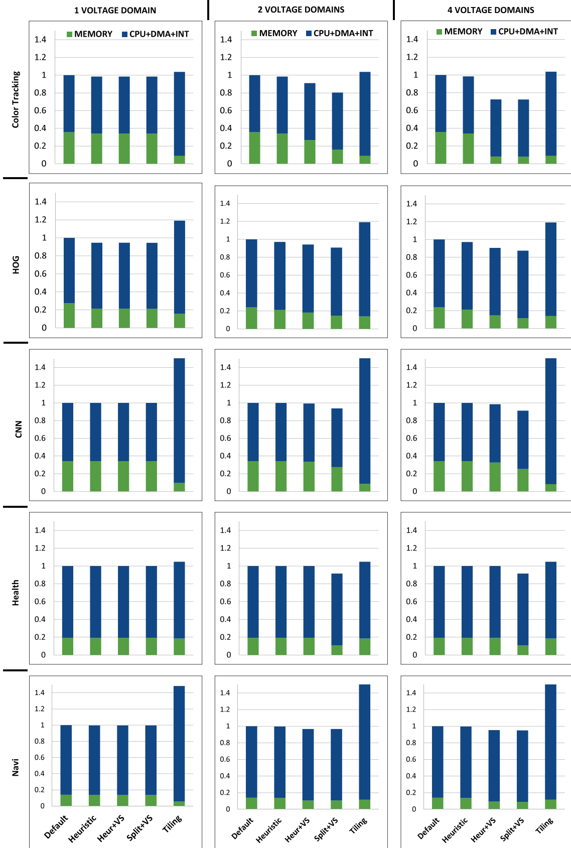
Fig. 11. Normalized energy consumption of the full SoC.
