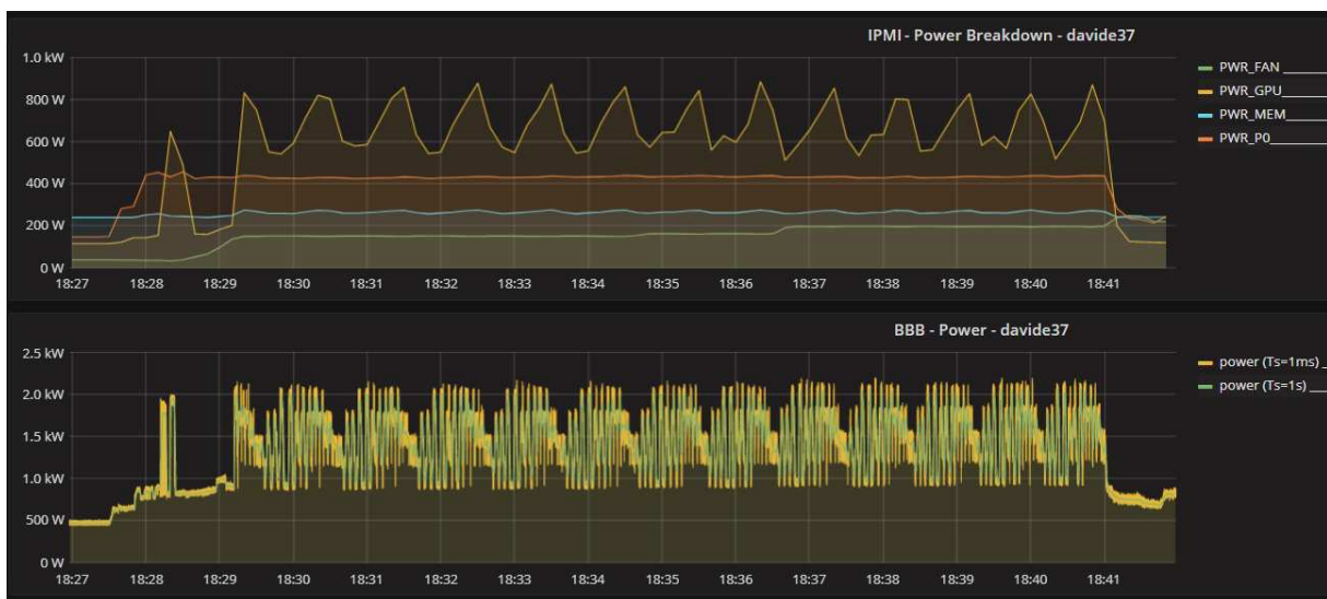
Figure 3: Grafana Snapshot on time windows of 15 minutes (18:27-18:42). OCC and IPMI Daemon per component power measurement (Top Plot) vs. Node Power Consumption Daemon (Bottom Plot).
