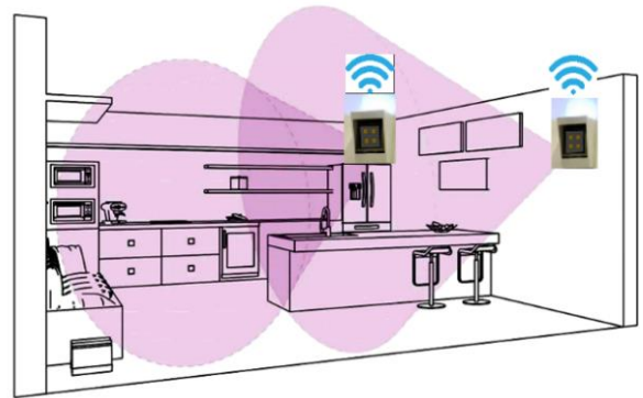
Fig. 1. Envisioned indoor scenario for people localization and tracking. In this case, two readers are present in the same room and can be embedded in everyday life objects and furniture (i.e., a wall lamp).
