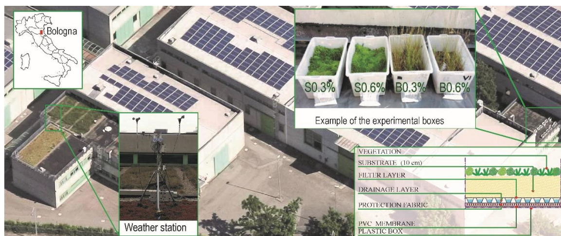
Figure 1. Aerial view of the experimental site showing: the location of the experimental test boxes, the position of the weather station and the stratigraphy of the green roof.
