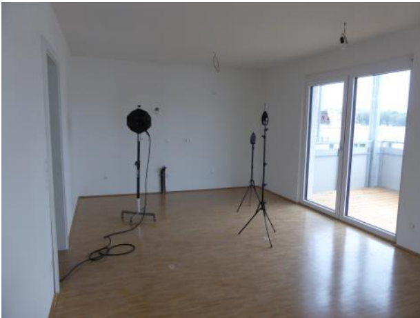
Figure 1: Measurement of sound insulation
