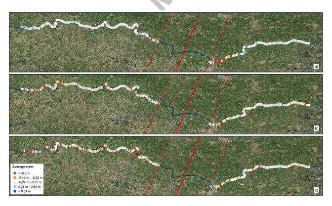
**Figure 13.** ME for all the points classified as interior water for (a) high , (b) mean and (c) low flow conditions.
