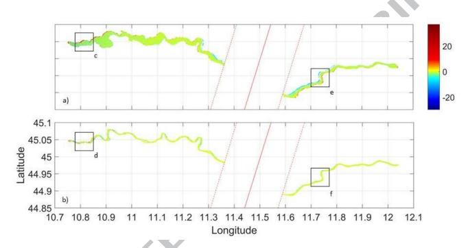
**Figure 8.** Errors (m) in water surface elevation sensed by SWOT at points classified as interior water under different flow conditions: (a) high and (b) low flows (panels (c), (d), (e) and (f) are reported in Figure 9).
