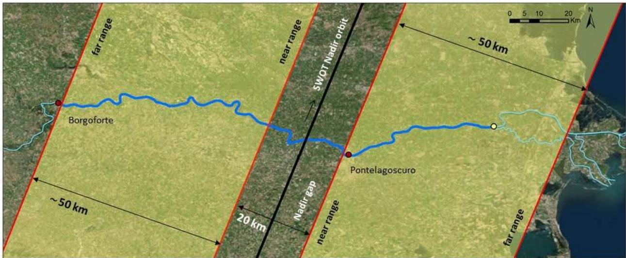
**Figure 2.** Example of a SWOT orbital pass over the study area: satellite swath (yellow areas), Po river reach considered in the study (dark blue; see also red box in Figure 1), flowing from the gauging station (red points) of Borgoforte to the beginning of the river delta (yellow point).
