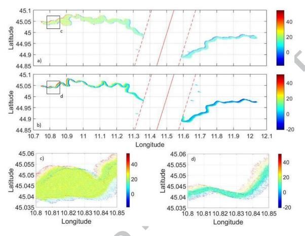
**Figure 6.** Pixel clouds showing the surface elevation (m a.s.l.) sensed by SWOT under different flow conditions, (a) high and (b) low flows, referring to all point classification; zoom in of panels (c) and (d) highlight the pixel clouds observed within a small river portion.
