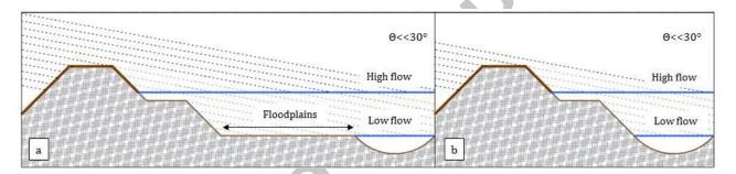
**Figure 4.** Layover illustration for embanked river in case of incidence angles <<30° and in case of (a) large or (b) absent lateral floodplains (modified from Fjortfot *et al.*, 2014). Dashed lines indicate constant range from the sensor; i.e. radar returns from the dashed line return to the sensor simultaneously.
