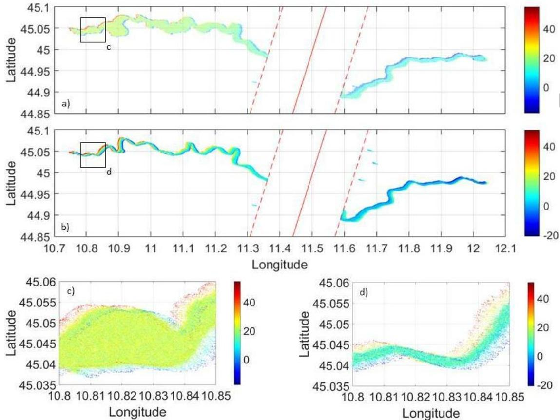
**Figure 6.** Pixel clouds showing the surface elevation (m a.s.l.) sensed by SWOT under different flow conditions, (a) high and (b) low flows, referring to all point classification; zoom in of panels (c) and (d) highlight the pixel clouds observed within a small river portion.
