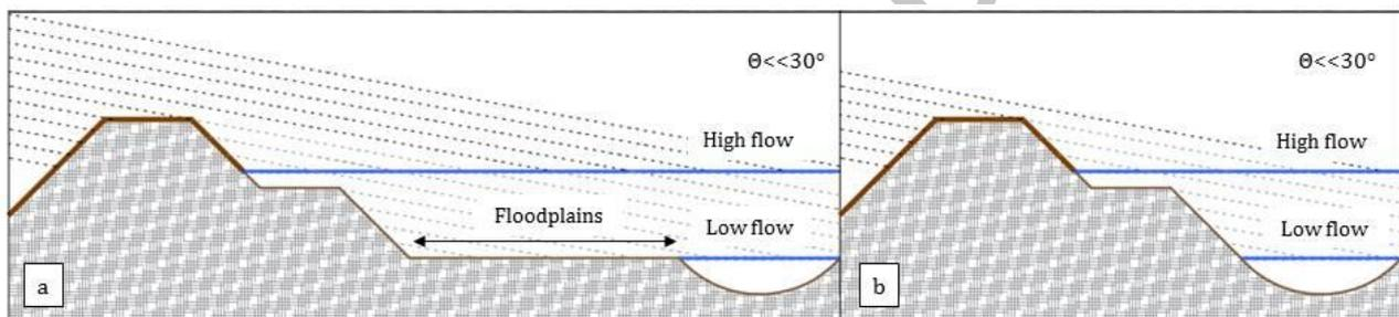
**Figure 4.** Layover illustration for embanked river in case of incidence angles  $\ll 30^\circ$  and in case of (a) large or (b) absent lateral floodplains (modified from Fjortoft *et al.*, 2014). Dashed lines indicate constant range from the sensor; i.e. radar returns from the dashed line return to the sensor simultaneously.
