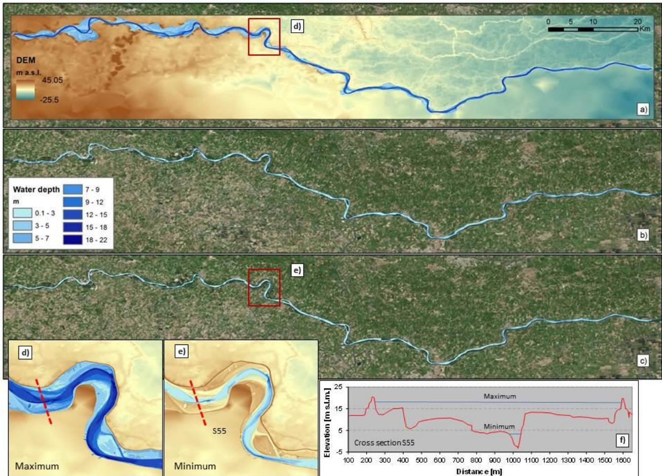
**Figure 3.** Input datasets for the SWOT simulator: 2D water depth coverage simulated for (a) high, (b) mean and (c) low river flow conditions (blue scale) and 2 m resolution DEM for river bathymetry and flood prone areas (from brown to green). Red boxes identify the same area used to show the different flood extents for (d) high and (e) low flow events, which may correspond to very different water depths at a given cross-section (e.g., cross-section S55; panel (f)).
