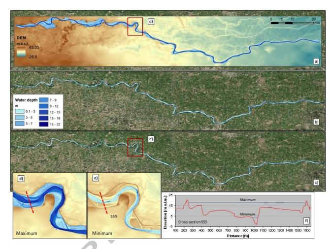
**Figure 3.** Input datasets for the SWOT simulator: 2D water depth coverage simulated for (a) high, (b) mean and (c) low river flow conditions (blue scale) and 2 m resolution DEM for river bathymetry and flood prone areas (from brown to green). Red boxes identify the same area used to show the different flood extents for (d) high and (e) low flow events, which may correspond to very different water depths at a given cross-section (e.g., cross-section S55; panel (f)).
