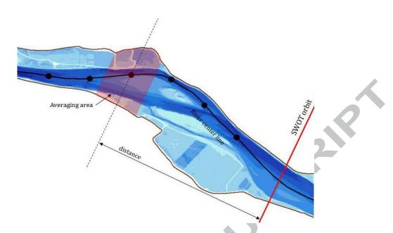
**Figure 5.** Schematic representation of the river discretization for the left swath; similar discretization has been adopted for the right swath.
