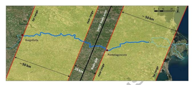
**Figure 2**. Example of a SWOT orbital pass over the study area: satellite swath (yellow areas), Po river reach considered in the study (dark blue; see also red box in Figure 1), flowing from the gauging station (red points) of Borgoforte to the beginning of the river delta (yellow point).
