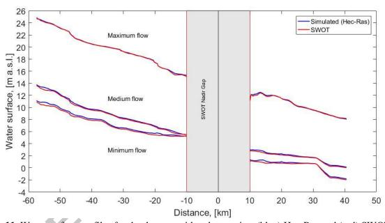
**Figure 11.** Water surface profiles for the three considered scenarios: (blue) Hec-Ras and (red) SWOT water profiles estimated considering an averaging area of 1 km<sup>2</sup> (see section 4.2) and a ten-point moving average filter.
