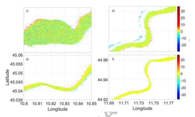
**Figure 9.** Errors (m) in water surface elevation at points classified as interior water under different flow condition: panels c) and e) refer to high flow, panels d) and f) refer to low flow (see boxes in Figure 8).
