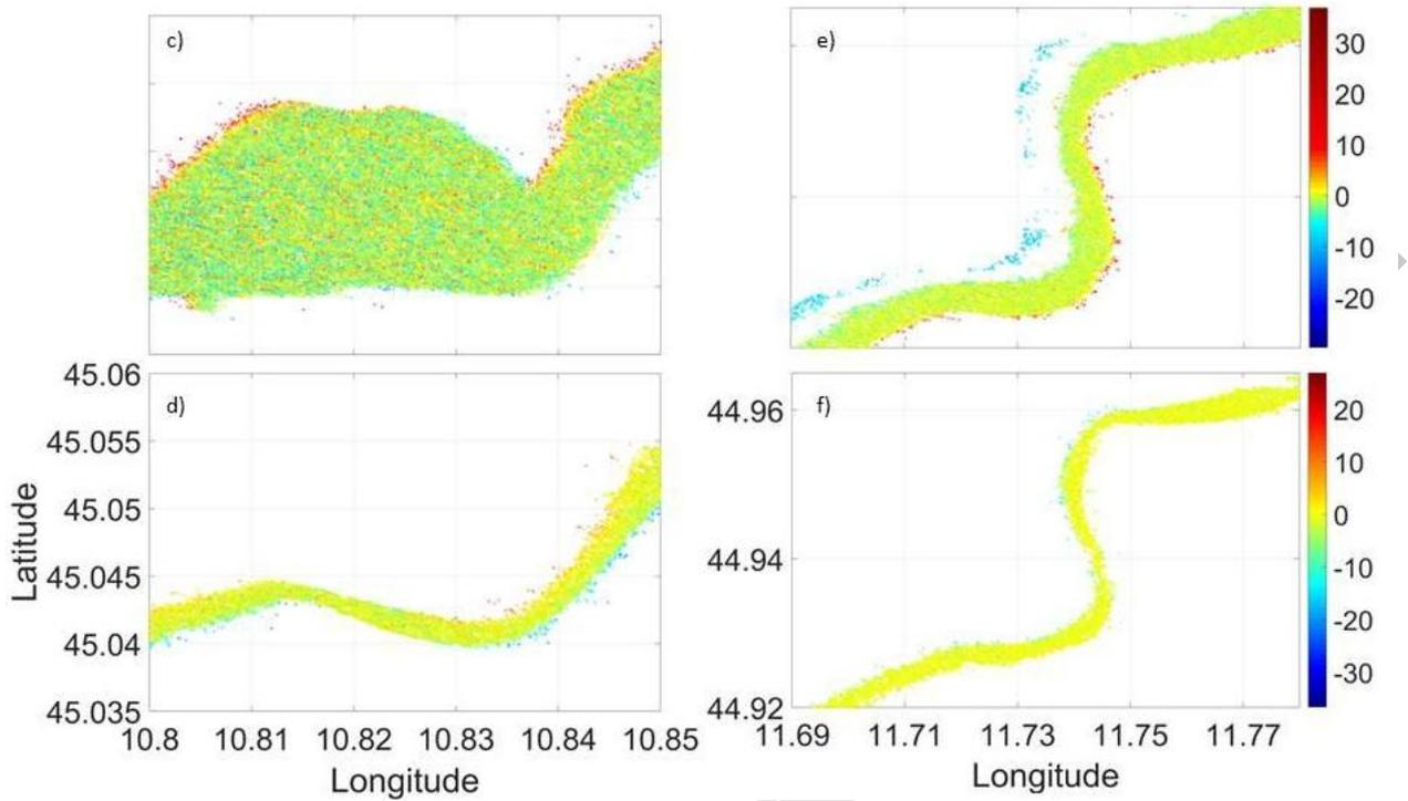
**Figure 9.** Errors (m) in water surface elevation at points classified as interior water under different flow condition: panels c) and e) refer to high flow, panels d) and f) refer to low flow (see boxes in Figure 8).
