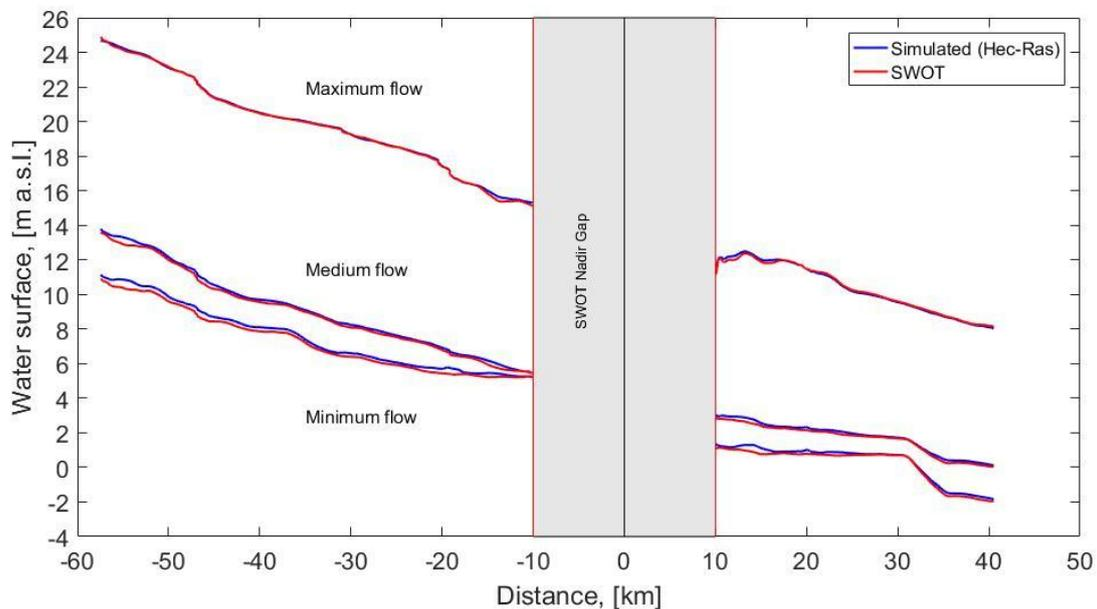
**Figure 11.** Water surface profiles for the three considered scenarios: (blue) Hec-Ras and (red) SWOT water profiles estimated considering an averaging area of  $1 \text{ km}^2$  (see section 4.2) and a ten-point moving average filter.
