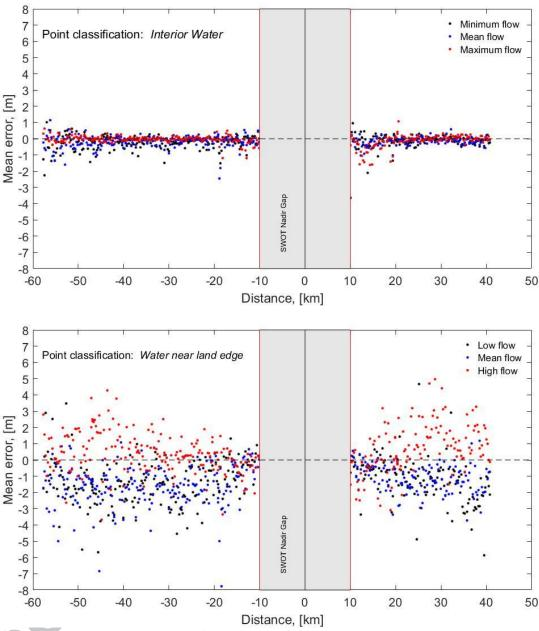
**Figure 12.** Mean error (ME) on water surface elevation for interior water (upper panel) and water near land edge (lower panel) points; points are shown in relation to the distance from the Nadir orbit (negative distances indicate the left swath).
