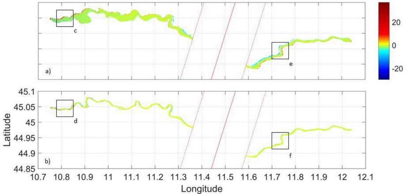
**Figure 8.** Errors (m) in water surface elevation sensed by SWOT at points classified as interior water under different flow conditions: (a) high and (b) low flows (panels (c), (d), (e) and (f) are reported in Figure 9).
