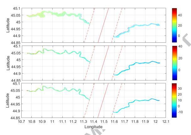
**Figure 7.** Pixel clouds reproducing the water surface elevation (m a.s.l.) for points classified as interior water under different flow conditions: high, mean and low flows (upper, intermediate and lower panel, respectively).
