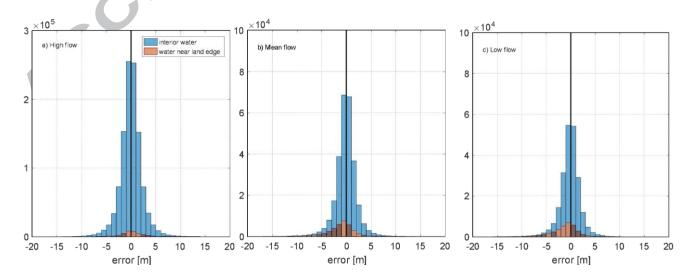
**Figure 10.** Histograms of errors,  $\varepsilon$ , on water surface elevation for the three scenarios considering points classified as interior water (blue bars) and water near land edge (brown bars).
