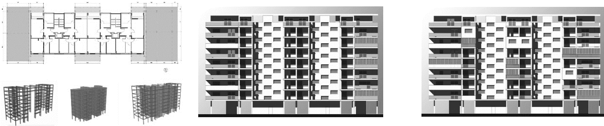
Figure 9. Structure frame for the T7 block type. Technical study of the structural feasibility to combine additions on the top and aside the buildings (and thus new residential units) with façade additions.
