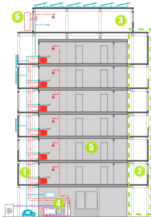
Figure 5. Exoskeleton providing existing building (5) with: strengthening by GET structure (2), energy saving and plant distribution (1, 4, 6) increased comfort and living areas for residents, and additional new units (3).
