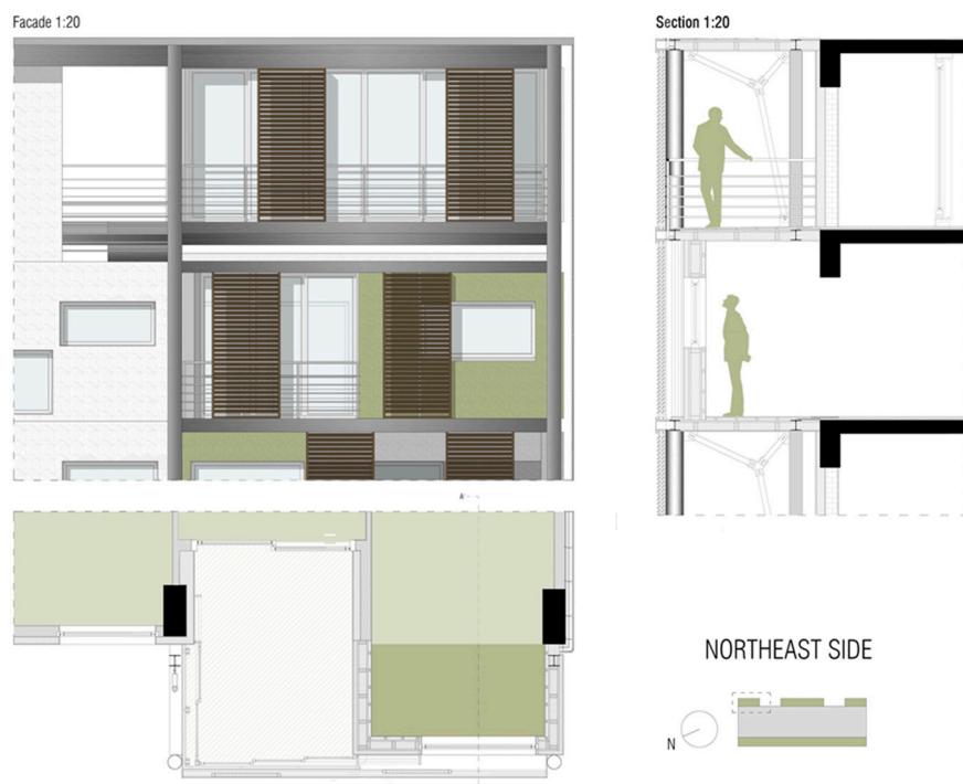
Figure 17. Façade, plan and detailed section of a typical application of the GET system on the Peristeri building.
