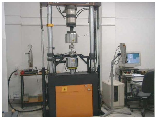
Fig. 5. Uniaxial loading tensile servo-hydraulic testing machine INSTRON® 1343
