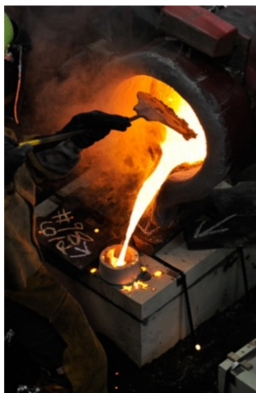
Fig. 1. Production of cast iron in laboratory
