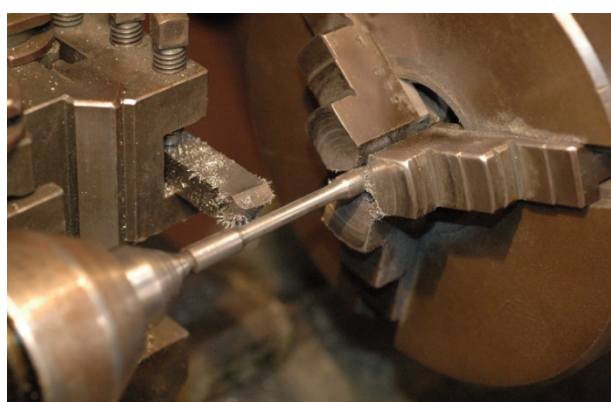
Fig. 6. "Dog bone" shape for a tensile specimen
