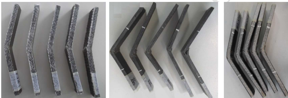
Figure 4 Flexural samples removed from different laminates and their mode of failure flax (left), basalt (centre), flax/basalt hybrids (right)
