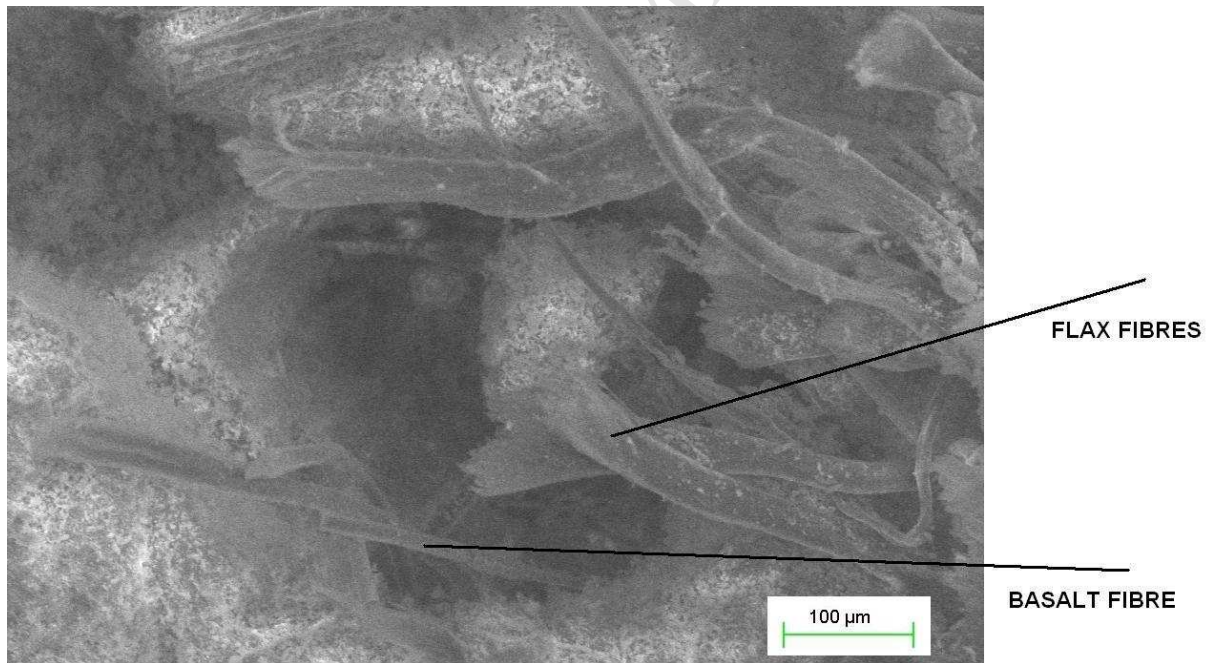
Figure 5c SEM observation following flexural fracture on flax-basalt hybrid laminates
