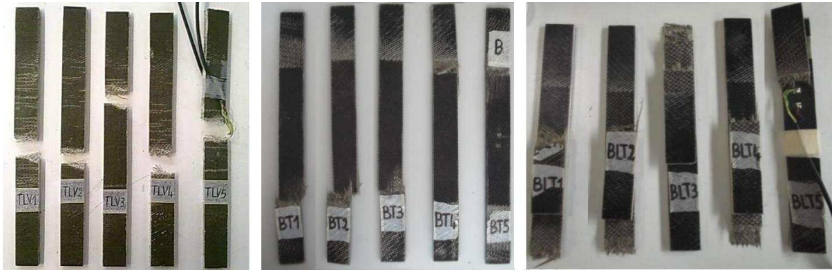
Figure 3 Tensile samples removed from different laminates and their mode of failure: flax (left), basalt (centre), flax/basalt hybrids (right)
