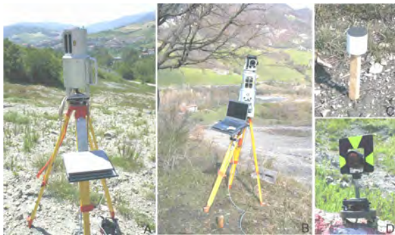
Figure 3. Instruments adopted for the Laser Scanning surveys: A) Riegl LMS-Z210; B) Riegl LMS-Z420i; C) Cylindrical Retroreflector (height 100 mm \times diameter 100 mm); D) Retroreflector prism used in the first campaign.
