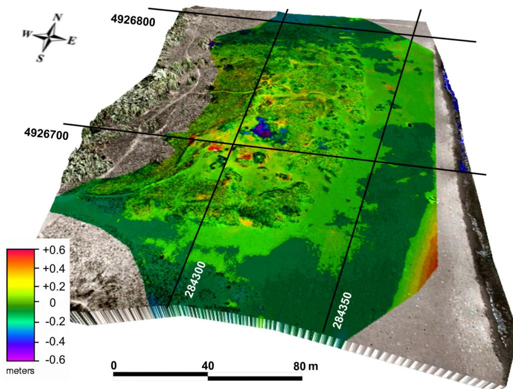
As can be seen from Figure 8, the elevation differences are almost neutral all over the investigated area (green tones) but, as seen in the point clouds comparison, where sudden changes on topographic
