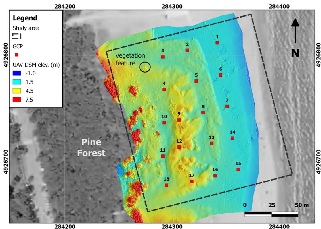
The meshed DSM shows a fine representation of the elevation dataset over the study area. Patches with elevations of over 7.5 m are known to represent vegetated areas. Consequently, such features were not included in the successive validation process or in the comparison with the DSM derived using TLS methodology. Meanwhile, features representing sparse and low (15 to 20 cm) vegetation
