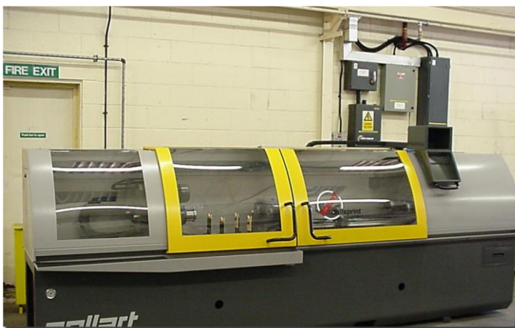
Figure 2. Use of rigid barriers in wood processing (Procter, 2015)
