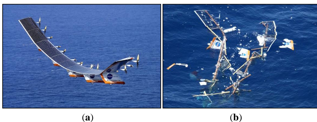
Figure 9. NASA's Helios wing (a) and its wreckage in the Pacific (b) (courtesy of NASA).
