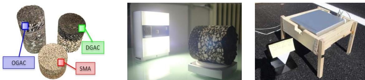
Some acquisition have also been performed directly on the paving site, in order to assess the applicability of this technique in all operating conditions, considering also the possibility to get repeated measures for future monitoring purposes. For the tests performed on-site, the pavement can be classified as SMA.
