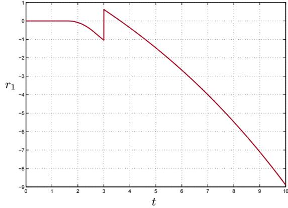
Fig. 8. Residual  $r_1$  with delayed saturated ramp at fault input  $u_1$  and sinusoid at input  $u_2$
