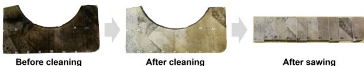
Figure 3. Naturally weathered slab, before and after cleaning, and “NAT” specimens.
