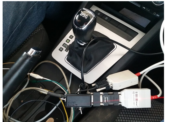
Fig. 5. CAN bus tapping. Note that both USB devices are connected to the same line by using the black T-connector.
