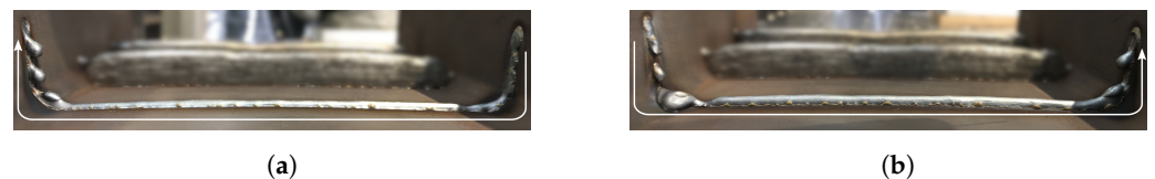
Figure 16. Two layers with slicing from outside to inside (a) Layer 1; (b) Layer 2.
