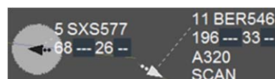
Fig. 12 Attention guidance elements for unattended aircraft (semi-transparent circle in automation level 0, "SCAN" in automation level 1)
