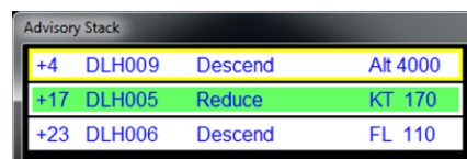
Fig. 17 Advisory stack lists "controller commands" that will be executed automatically
