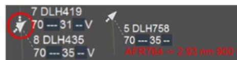
Fig. 13 Attention guidance elements for conflicting aircraft (red circle around conflict partners in automation level 0, otherwise red alpha-numeric values)
