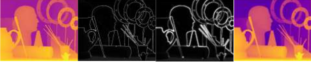
Fig. 3: High-frequency information loss (factor 4 \times ) . From left to right, HR depth map and its corresponding gradient map, followed by the gradient map from bicubic upsampled LR depth map and LR depth map itself. HF information is mostly lost in the second gradient map.
