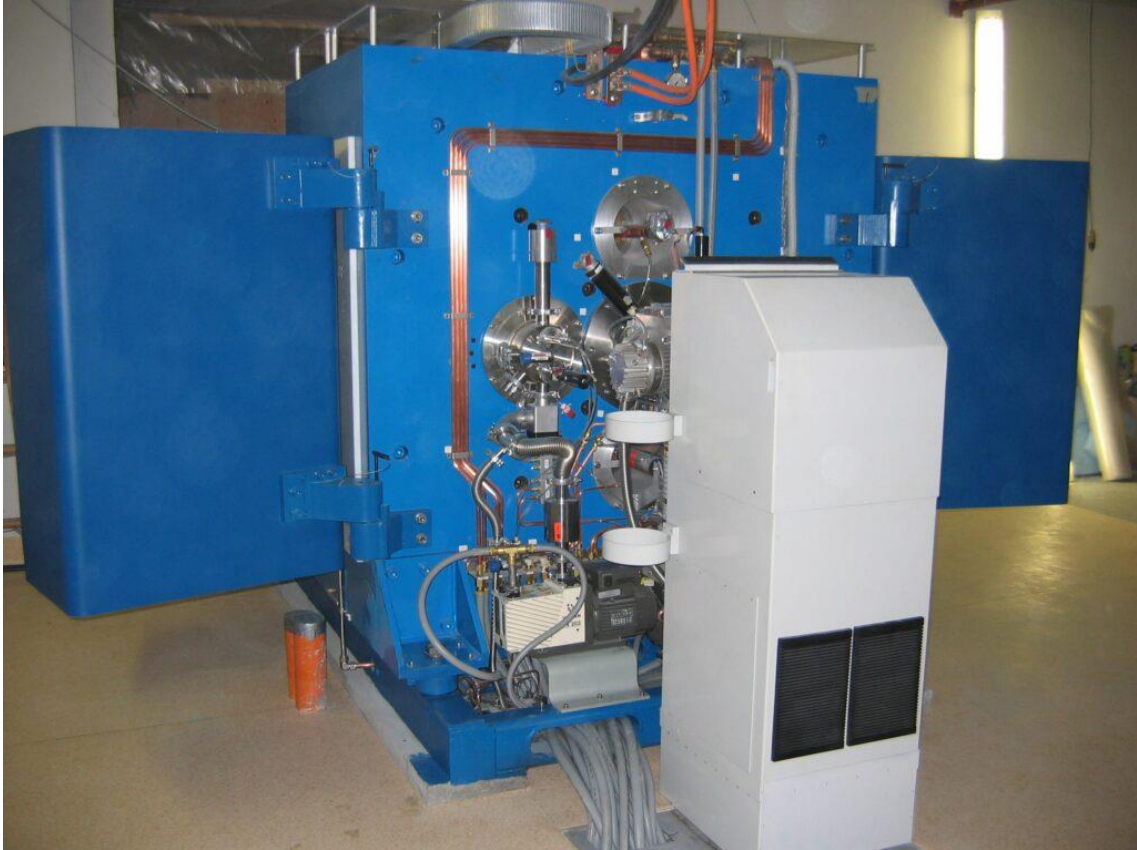
Figure 3. The ACSI TR-19 cyclotron , shown in a configurations with local shields on the target stations. Courtesy of mr. B. Kovacs.
