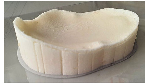
Fig. 5 PCU cranial plate printed by APF with 50% support density
