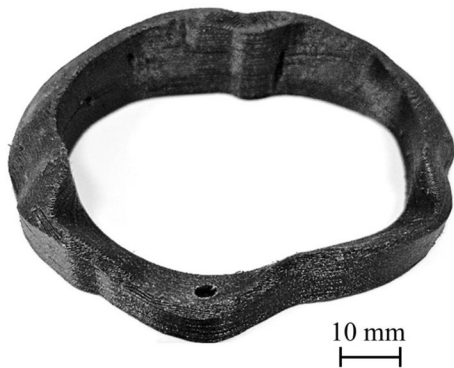
Fig. 3 Support base used to anchor the cranial plate for testing
