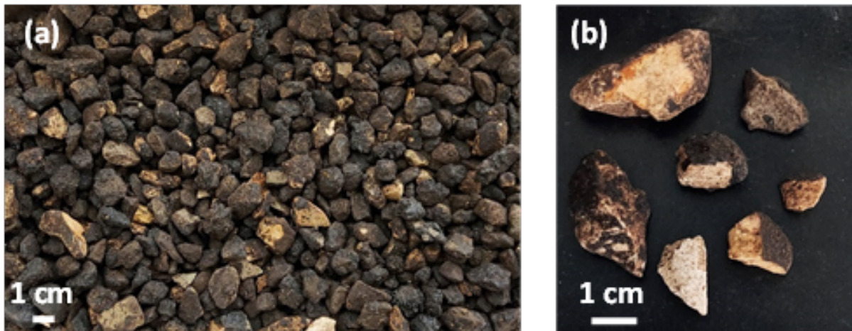
Figure 6: Images of (a) AN RAP and (b) a detail of RAP after freeze-thaw cycles in presence of NaCl solution.
