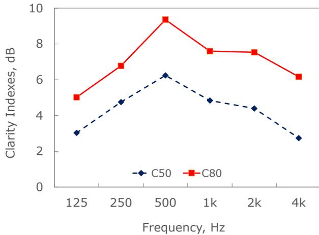
Fig. 4. Measured results of clarity indexes (C<sub>50</sub> and C<sub>80</sub>).
