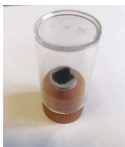
Figure S6 Photographs of sealable SEM holder for sample transfer.
