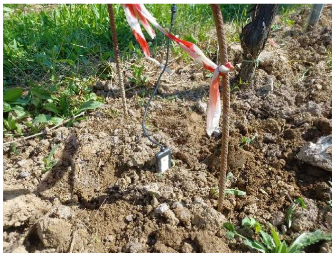
Figure 3. Probe inserted into sandy soil during the field experiment.
