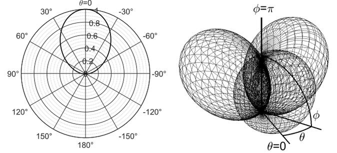
**Fig. 1.** Horizontal polar pattern of a fourth order cardioid (left). 3-dimensional plot of the 3DVMS virtual microphones aiming at directions  $(\vartheta = 0^\circ; \varphi = 45^\circ)$ ;  $(\vartheta = 120^\circ; \varphi = 45^\circ)$ ;  $(\vartheta = -120^\circ; \varphi = 45^\circ)$  (right).
