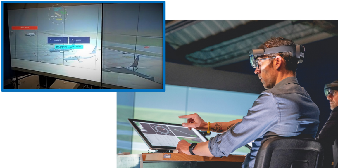
Figure 2 – The ATCOs can contemporarily see both the out of the tower view and the Augmented Reality Overlays through HoloLens2. The personal view of the user during the V/A-R Air Gestures HMI interaction validation exercise is depicted in the blue square.
