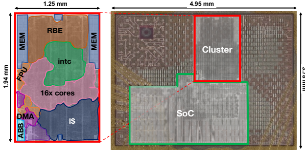
Fig. 6. Microphotograph of the MARSELLUS prototype fabricated in GlobalFoundries 22FDX technology.
