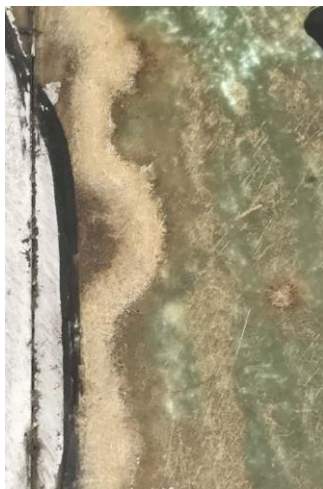
Fig. 12 a) Fibers emerging from fibreglass inside the dome; b) local bulge on the internal surface of the dome.
