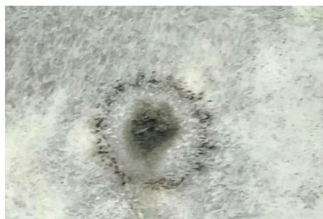
Fig. 12 a) Fibers emerging from fibreglass inside the dome; b) local bulge on the internal surface of the dome.
