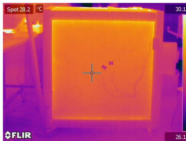
Figure 9. Thermal image of the contour of the exterior surface temperature T_{se} , obtained with a thermal camera, in a generic instant of the test on the high conductance sample.
