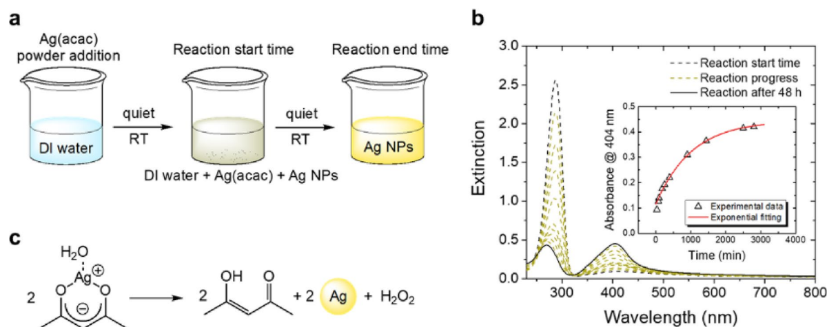
Fig. 1. AgNP synthesis. (a) Schematic representation of the synthesis process of AgNPs using Ag(acac). (b) Extinction spectra of the solution acquired at regular intervals, illustrating the progression of the reaction. The inset shows the kinetic profile of AgNP growth. (c) Proposed mechanism for AgNP synthesis.
