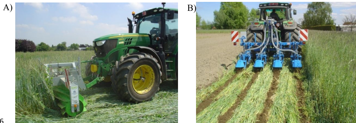
146 147 Picture 5. Machinery used for NT-RC management at the INAGRO (BE-INAGRO) organic farm station. A - Roller 148 crimper; B - In-line tiller.
