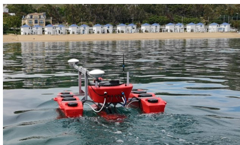
Fig. 2 - OpenSWAP in operation with a Klein Hydrochart 3500 multibeam installed between the two hulls.
