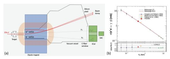
Fig. 100 a The PADME detector layout. The gamma gamma detection technique is also highlighted. b Status of  $e^+e^- \to \gamma\gamma$  cross-section measurements
