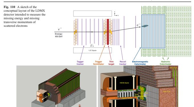
Fig. 111 Left: an overview of the LDMX detector solid model. Right: a cutaway overview of the LDMX detector showing, from left to right, the trackers, trigger scintillator and target inside the spectrometer dipole, the ECal, and the Side and Main HCal
