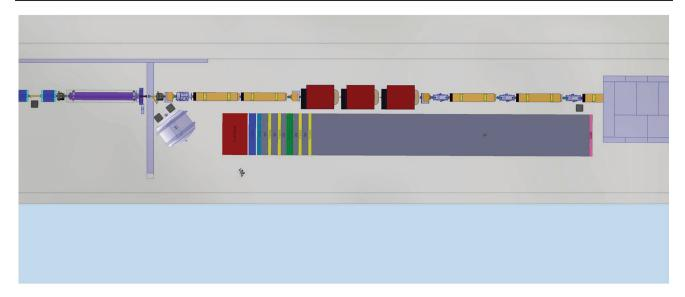
Fig. 93 Top view of the SHADOWS detector in the experimental hall. The beam is entering from right to left. The shielded area containing the TAXes dump is visible at right. SHADOWS detector is sketched at the bottom of the figure. The dimensions of the detector and the beamline elements are to scale
