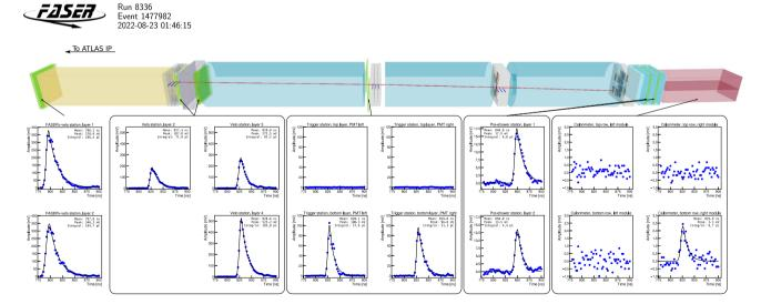
**Fig. 78** FASER Event Display of a muon travelling through the length of the FASER detector during 2022 proton-proton collisions. The waveforms below the display are the reconstructed PMT ADC pulses of the
