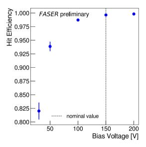
**Fig. 81** The SCT hit efficiency versus the applied bias voltage (in volts) is shown. The nominal setting of 150 V is indicated by a dashed line, and yields an average hit efficiency across the full tracker of  $99.64\pm0.10\%$ . These plots used data taken in dedicated FASER runs, where the tracker settings were changed from nominal, during LHC collisions in July 2022
