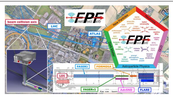
**Fig. 84** Location and layout of the Forward Physics Facility. The FPF will be located along the beam collision axis about 620 m west of the ATLAS interaction point and is envisioned to be 65 m long and 8.5 m
