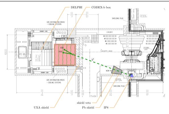
Fig. 66 Top view of the LHCb cavern UX85 at point 8 of the LHC, overlaid with a top view schematic of the CODEX-b detector. Adapted from Ref. [1030]
