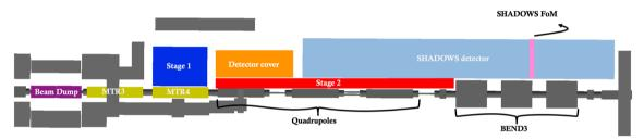
**Fig. 94** The optimized SHADOWS setup including the MIB system. The muons created in the beam dump (purple) are pushed off-axis by the MTR3 (B1) and MTR4 (B2) magnet (yellow) to reduce the muon back-
