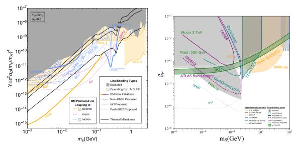
**Fig. 59** Left: reach of past, present, and future experiments on dark photon-mediated dark matter production [834]. Thermal milestones are shown as black solid lines. Right: reach of past, present, and future experiments on a muon-philic scalar that can address the  $(g-2)_{\mu}$
