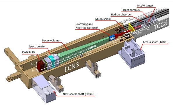
Fig. 95 Overview of the BDF/SHiP experimental setup in the SPS ECN3 beam facility
