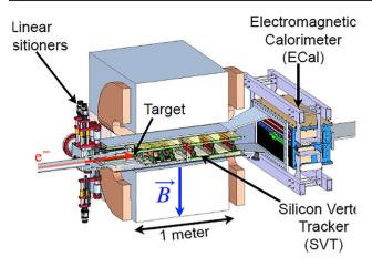
Fig. 105 The HPS detector
