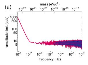
**Fig. 32** a Upper 95% confidence limits on the oscillation amplitude  $b_{\rm up}(\omega)$  of the antiproton Larmor frequency. **b** 95% confidence limits on the axion-antiproton interaction parameter as a function of the axion mass. The grey area shows the parameter space excluded by axion emission from antiprotons in SN 1987A. The dark blue area shows
