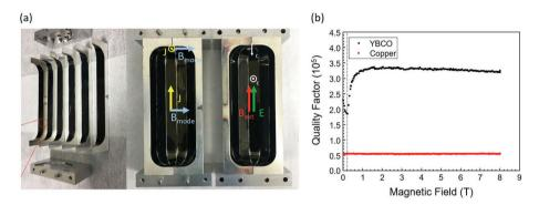
Fig. 22 a Photo of CAPP's prototype superconducting cavity. **b** Q-factor measurements of CAPP's 1st generation prototype superconducting cavity. These are imported from figure 1, 4 of [284]
