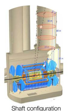
**Fig. 64** The two ANUBIS configurations considered in the sensitivity study: the original shaft configuration where four tracking stations are placed in the main PX14 shaft of ATLAS, and the ceiling configuration,
