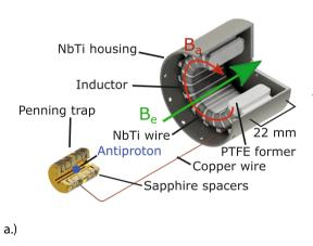
Fig. 33 a Superconducting toroidal resonator connected to a Penning trap. The green arrow indicates the external magnetic field of the superconducting magnet, the red arrow indicates the magnetic field sourced
