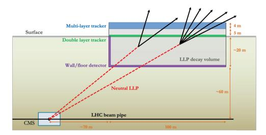
Fig. 68 MATHUSLA geometry relative to the CMS collision point, illustrating how LLPs can decay in the detector and be reconstructed as displaced vertices by the trackers. For clarity, the modular structure of the MATHUSLA detector is not shown
