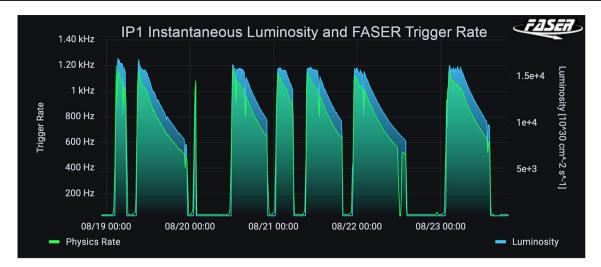
**Fig. 82** The instantaneous luminosity measured at Interaction Point 1 (blue) and the FASER total trigger recorded rate (green) are shown for 8 LHC fills between August 19th to 23rd, 2022. The trigger rate trend generally follows the luminosity trend but it is evident that the trigger rate falls off more strongly at the beginning of fills than the luminosity.
