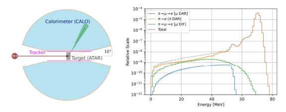
Fig. 144 Sketch of the apparatus (left). Typical calorimeter energy spectrum for  $\pi^+ \to e^+$  and  $\pi^+ \to \mu^+ \to e^+$  processes, after background suppression. Note  $\pi^+ \to e^+$  the low energy tail (right). DAR refers to decay-at-rest and DIF stands for decay-in-flight
