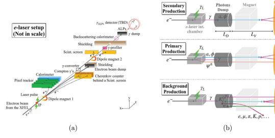
Fig. 97 e-laser experimental setup (a) and signal and backgrounds productions in LUXE-NPOD (b). The secondary signal production happens with the interaction of the photons in the physical dump material, with
