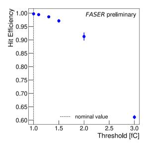
**Fig. 80** The SCT hit efficiency versus the applied hit threshold (in fC) is shown. The nominal threshold setting of 1 fC is indicated by a dashed line, and yields an average hit efficiency across the full tracker of  $99.64 \pm 0.10\%$ . This plot used data taken in dedicated FASER runs, where the tracker settings were changed from nominal, during LHC collisions in July 2022
