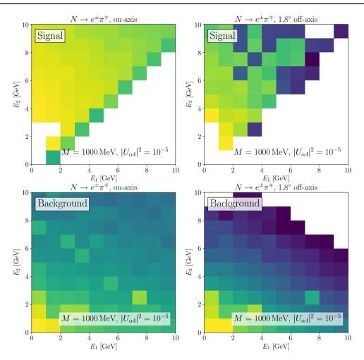
**Fig. 140** Two-dimensional distributions of signal events (top) and background events (bottom) in the plane spanned by the energies of the two HNL decay products. The large differences in the distributions help to suppress backgrounds. Panels on the left are for an on-axis
