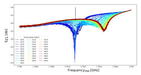
Fig. 19 Two-tone spectra measurements at frequency 7.74 GHz. First-tone through-transmission (S21) vs VNA-frequency dependencies recorded at different powers of the second-tone signal of frequency of 7.743 GHz applied to the Port 3
