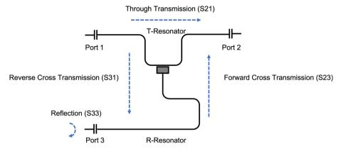
Fig. 18 Scheme of the T-type device composed of two resonators T and R coupled by a SQN (gray box)
