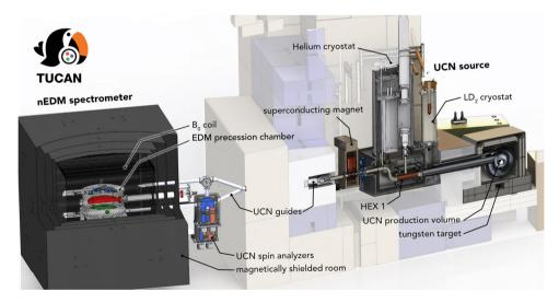
Fig. 26 Schematic diagram of the TUCAN EDM experiment. The major portion of the biological shielding is not shown. Protons strike a tungsten spallation target. Neutrons are moderated in a volume of  $LD_2$  cooled by the  $LD_2$  cryostat. They become UCN in a UCN production volume containing He-II, which is cooled by a helium cryostat. The
