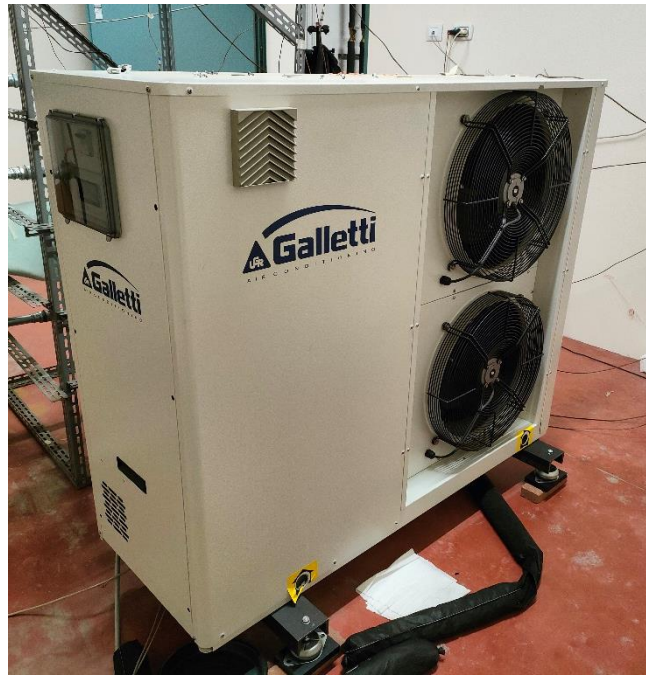
308 Figure 7. Heat pump inside the climate chamber (prototype based on mod. HWMC 010 309 HM).
