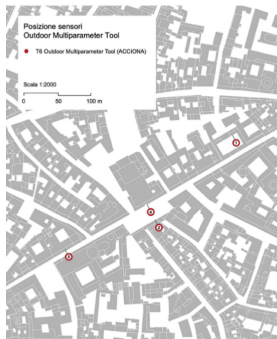
Figure 4. Location of ACCIONA outdoor sensors in Via Zamboni—Bologna. Sensors used for calibration are 1 and 4.
