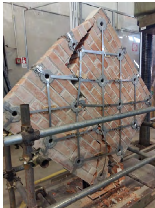
Figure 27. The failure mode of specimen M2-45.
