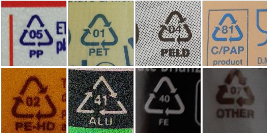
Figure 1: Some examples of recycling symbols in use in the European Union (European Commission, 1997). Minor graphical differences exist in the symbols introduced by other regulatory bodies. For instance, in the United States of America (ASTM International, 2021), the chasing arrows symbol is represented as a solid triangle.
