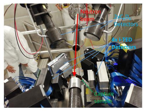
**Figure 7.** Photograph of the experimental setup at CERN's n\_TOF EAR1, for detector commissioning measurements in 2021. The sample is surrounded by two state-of-the-art C-fibre  $C_6D_6$  detectors and four i-TED Compton modules developed in the HYMNS ERC project [89].
