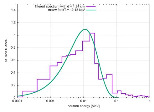
**Figure 8.** Preliminary results of simulations for the neutron energy distribution attainable at the NEAR station using a 30 cm thick aluminium fluoride moderator and a thin (1.34 cm) boron filter [92]. See text for details.
