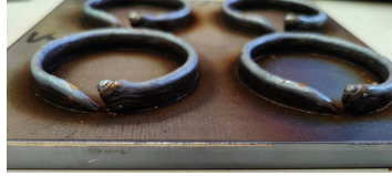
Fig. 6. Printing failure with low WFR.
