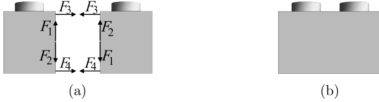
Figure 4: Two horizontally adjacent voxels. By adding forces between the voxels in (a), we model the brick shown in (b).
