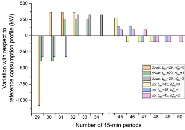
Fig. 3. Flexibility margins and corresponding recoveries of scenario 56 of PL A: down flexibility starting at  $t_{flex}=29$  (7:15 am) and up flexibility starting at  $t_{flex}=45$  (11:15 am).
