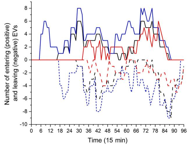
Fig. 1. Day-ahead forecast profiles of the number of EVs entering (solid lines) and exiting (dashed lines) in the three parking lots considered: PL A in black, PL B in blue, PL C in red.
